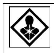
Severe Chronic Hazard
